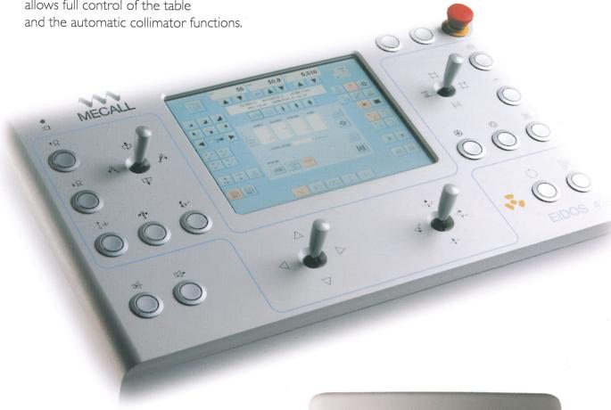
The operator remote console integrates the tilting table controls as well as the generator and image processor ones.
